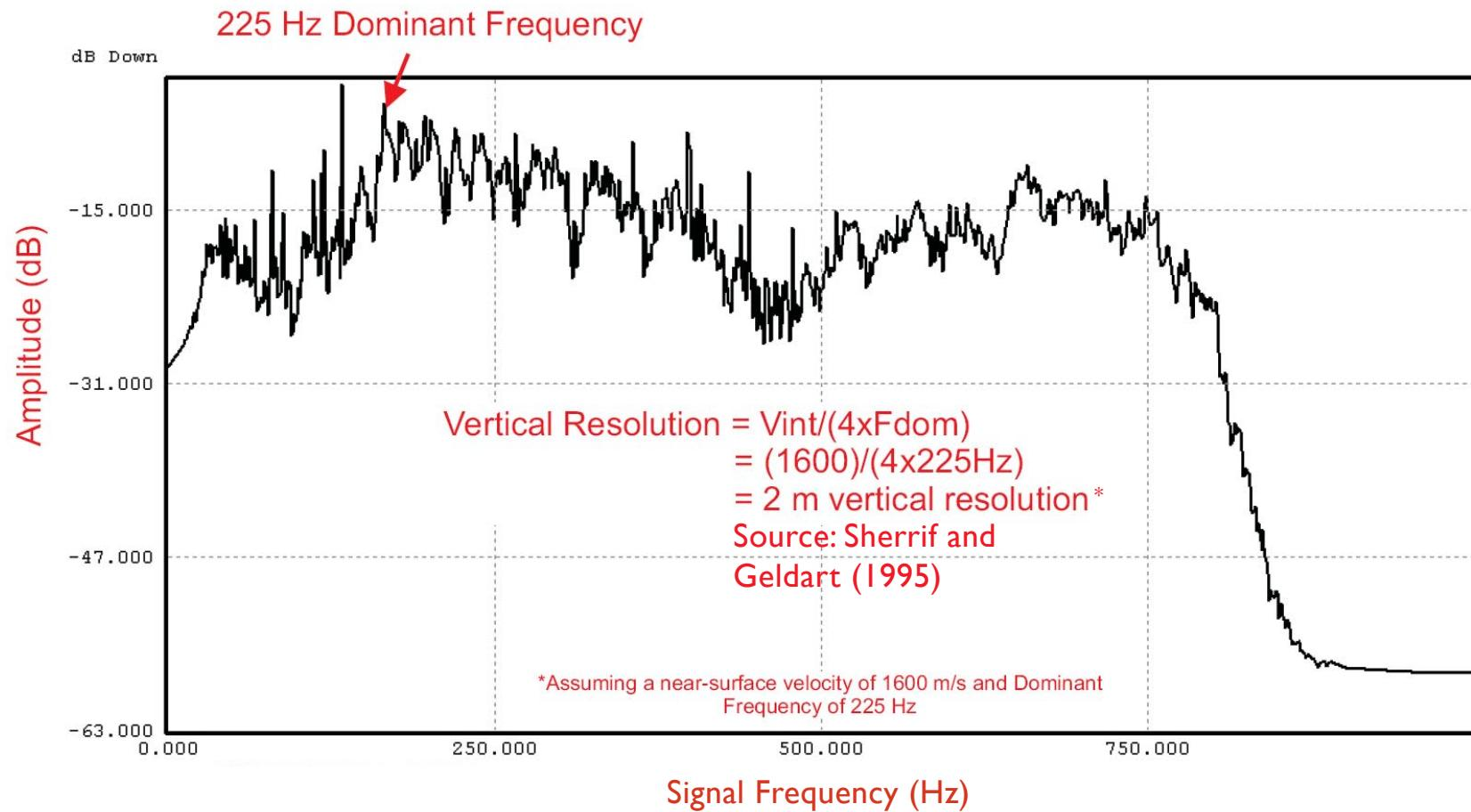
Frequency spectrum from 3D/2D seismic-reflection dataset showing dominant (fundamental) frequency of 200-225 Hz and calculated using 1600-1650 m/s to determine vertical resolution (2.00-2.06 and 1.78-1.83 m)
